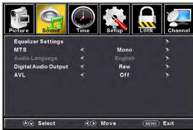
1. Press “▼” button to select “Equalizer Settings” and press the “ENTER/▶” button to enter sub-menu.
