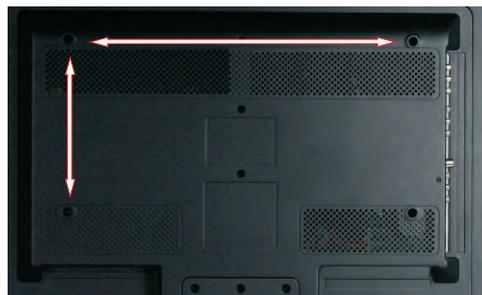
Mounting Specification : **400mm x 200mm** using screw size **M6**. Length of screw should not exceed **8mm**. Please Note : The **8mm** length of screw refers to how deep the screw can go inside the mounting holes. When you're buying screws, you should add the original 8mm to the thickness of your mounting plate in order to get the total screw length.
