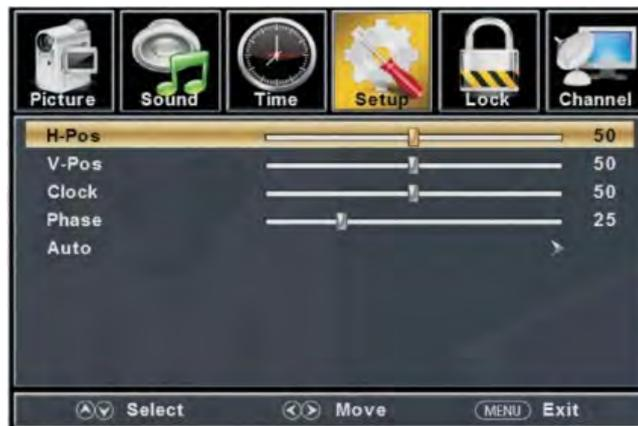
1. Press “▲/▼” button to select “H-Pos” and press the “◀/▶” button to adjust.
